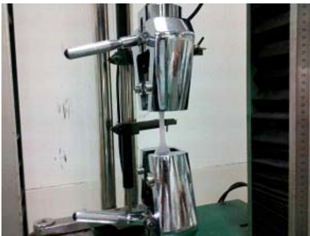
▲拉力試驗彈性及伸張力 (plasticity & elasticity)
