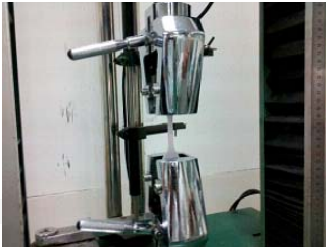
▲拉力試驗彈性及伸張力 (plasticity & elasticity)
